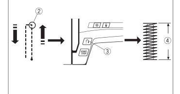
Tacking is used to reinforce pockets, crotches and belt carriers where extra strength is needed.
