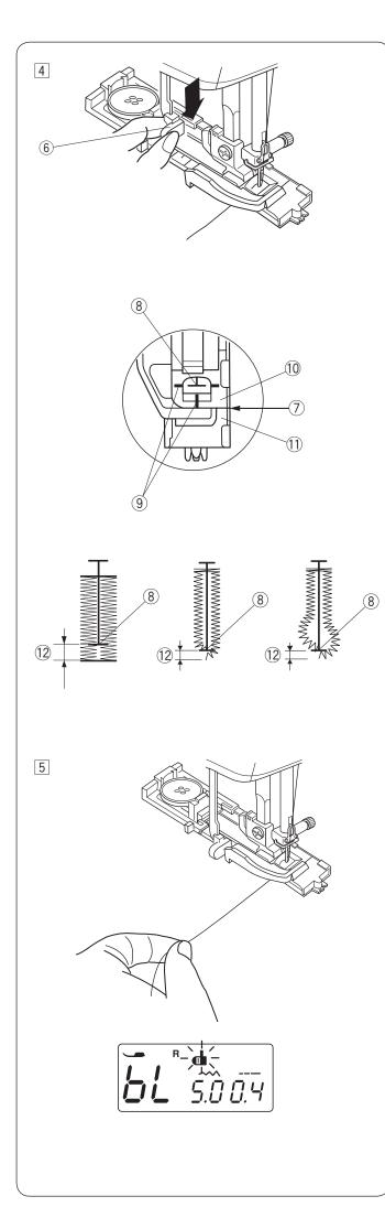
4 Lower the presser foot and pull the buttonhole lever down as far as it will go.
